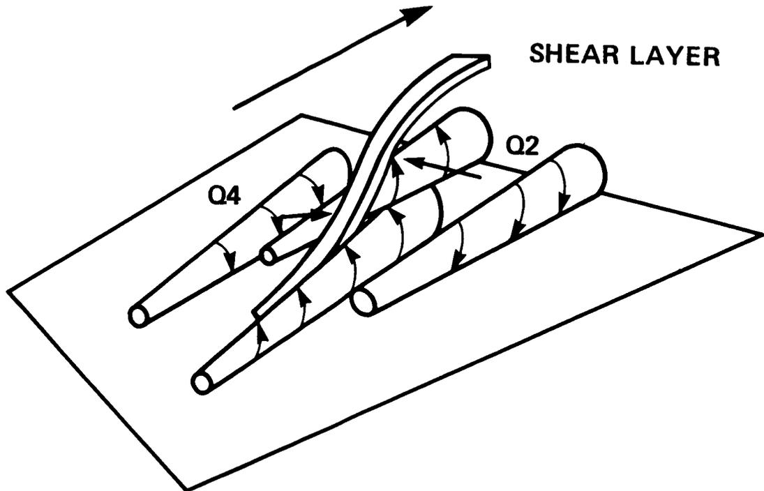
FIGURE 15. Sketch of the three-dimensional structure associated with the  $Q4/Q2$  event.
