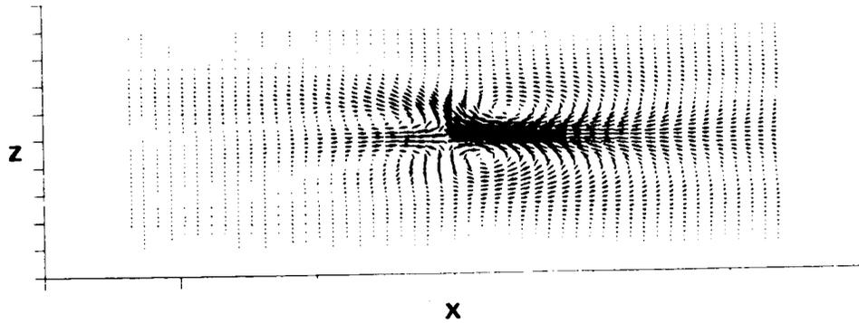
FIGURE 16. Linearly estimated  $(u, w)$  vectors in the  $x$ - $z$  plane passing through  $x_1$  given the  $Q4$  event at  $x_1$  and the  $Q2$  event at  $x_2$ .
