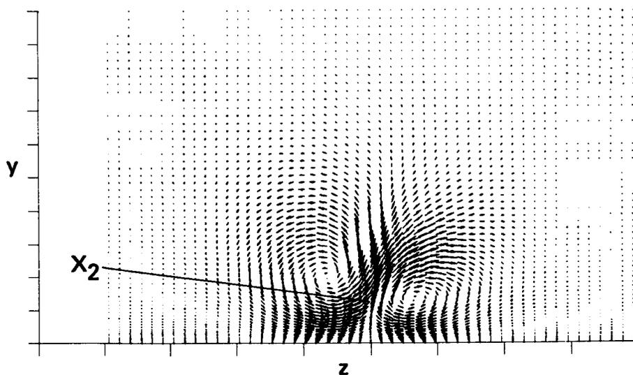
FIGURE 14. Linear estimate of  $(v, w)$  in the  $y$ - $z$  plane passing through  $x_2$  given the  $Q4$  event at  $x_1$  and the  $Q2$  event at  $x_2$ .
