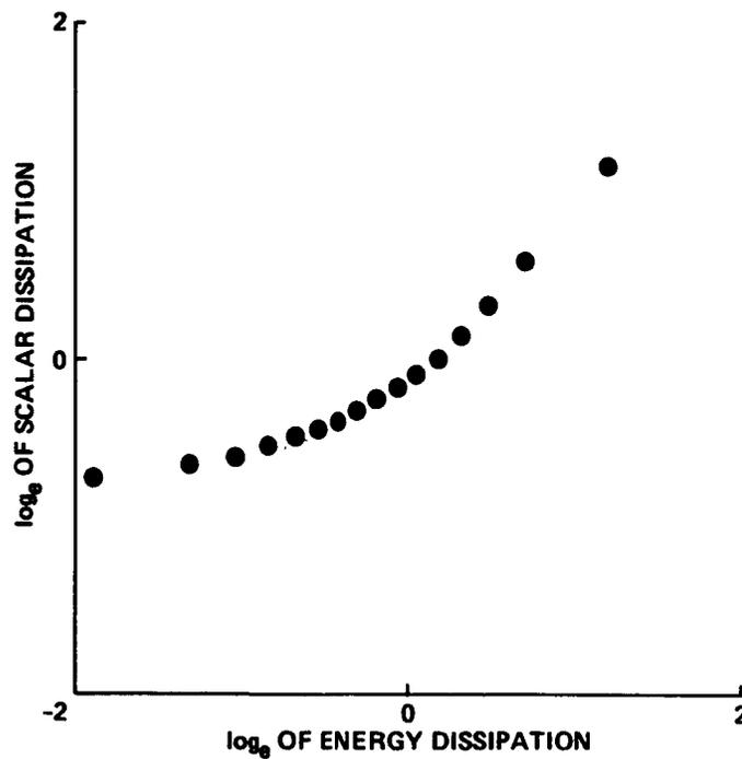
FIGURE 3. Mean scalar dissipation ( $D\nabla T \cdot \nabla T$ ) conditioned on energy dissipation reveals a changing power-law dependence.
