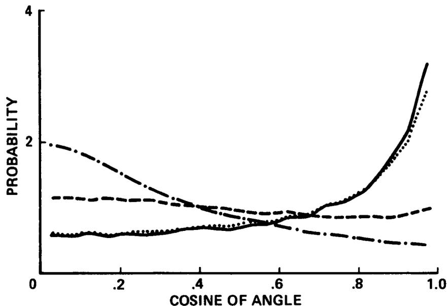
FIGURE 1. Pdf of the cosine of the angle between the vorticity and the principal strain-rate directions. ----  $\omega \cdot \alpha$ , .....  $\omega \cdot \beta$ , -.-  $\omega \cdot \gamma$ , —  $\omega \cdot \beta$  for  $\beta > 0$ . Note the increased probability for alignment with the intermediate strain-rate,  $\beta$ .
