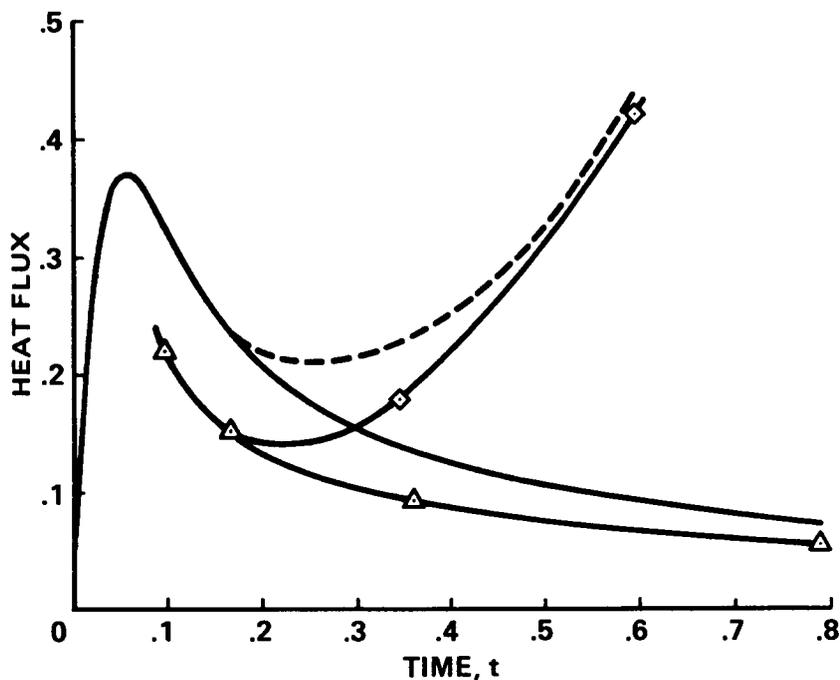
FIGURE 4. Comparison between the heat flux from the numerical simulations and that predicted by the model developed in Rogers, Moin & Reynolds (1986). — simulation  $g=0$ , ---- simulation  $g=30$ ,  $\triangle$  model  $g=0$ ,  $\diamond$  model  $g=30$ .
