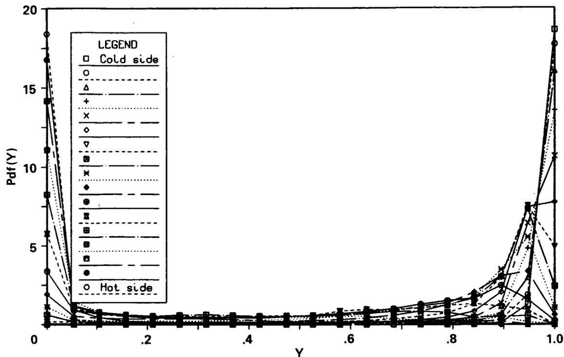
FIGURE 7. PDF of the mean reactant mass fraction.
