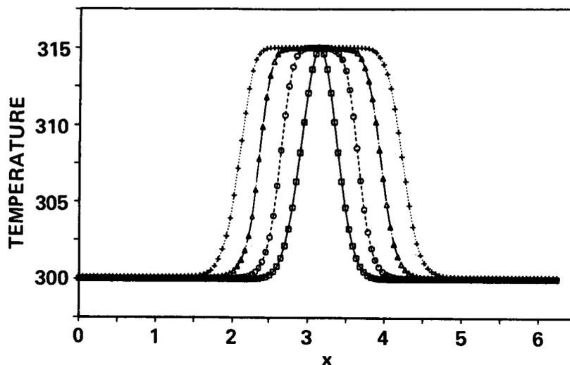
FIGURE 10. Mean turbulent temperature profiles at 200 step intervals.
