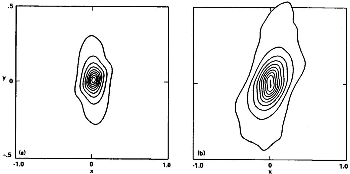
FIGURE 3. Comparison of velocity-velocity and velocity-scalar correlations in a homogeneous shear flow with a vertical mean temperature gradient. Note compressed x-scale. (a)  $x$ - $y$  plane,  $u_2u_2$  and (b)  $x$ - $y$  plane,  $u_2\phi$ .
