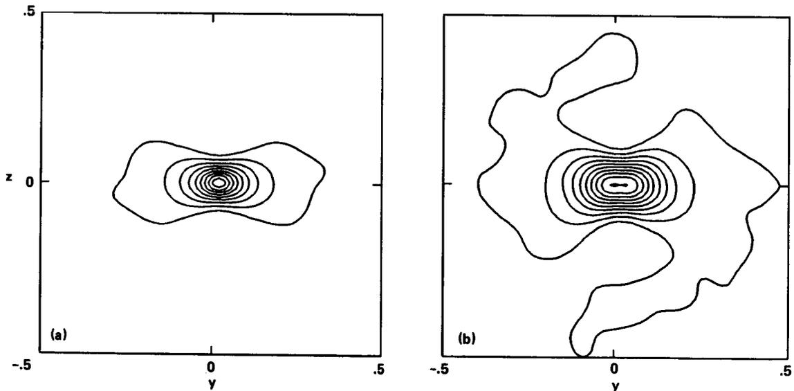
FIGURE 4. Comparison of velocity-velocity and velocity-scalar correlations in a homogeneous shear flow with a vertical mean temperature gradient. (a)  $y$ - $z$  plane,  $u_2u_2$  and (b)  $y$ - $z$  plane,  $u_2\phi$ .
