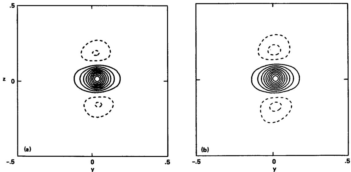
FIGURE 2. Comparison of velocity-velocity and velocity-scalar correlations in a homogeneous shear flow with a vertical mean temperature gradient. (a)  $y$ - $z$  plane,  $u_1 u_1$  and (b)  $y$ - $z$  plane,  $u_1 \phi$ .
