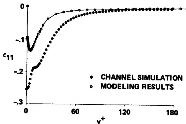
FIGURE 2. Distribution of dimensionless dissipation rate in  $\overline{uu}$  equation.
