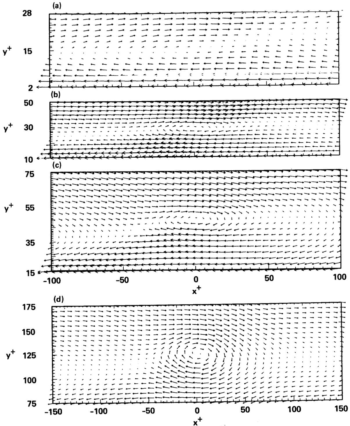
FIGURE 1. Educed velocity vector patterns in  $(x, y)$ -plane: (a) Centered at  $y^+ = 15$ ; (b)  $y^+ = 30$ ; (c)  $y^+ = 50$ ; (d)  $y^+ = 125$ . Note that the  $y$ -scales are stretched at different factors for each figures.
