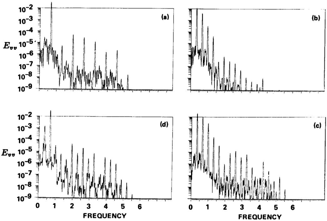
FIGURE 2. Time spectra at  $x = 28.1$  and  $y = 0$ . a) Case 1, forcing the fundamental only. b) Case 2, forcing the subharmonic only. c) Case 3, forcing the fundamental and its subharmonic with  $\phi = 0^\circ$ . d) Case 4, forcing the fundamental and its subharmonic with  $\phi = 90^\circ$ .
