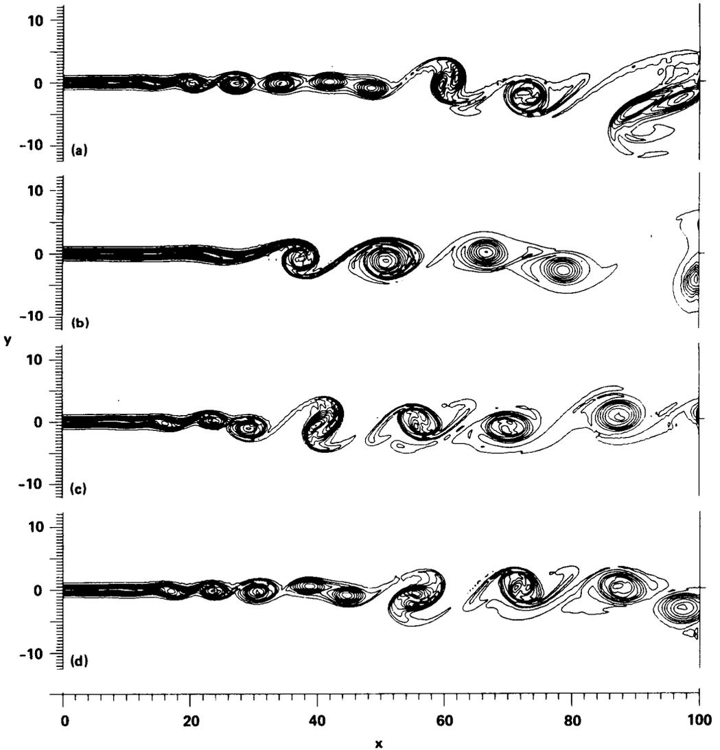
FIGURE 1. Contour plots of vorticity. a) Case 1, forcing the fundamental only. b) Case 2, forcing the subharmonic only. c) Case 3, forcing the fundamental and its subharmonic with  $\phi = 0^\circ$ . d) Case 4, forcing the fundamental and its subharmonic with  $\phi = 90^\circ$ .
