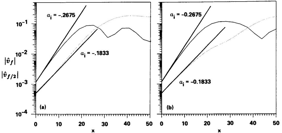
FIGURE 7. Development of  $|\hat{v}_f|$  and  $|\hat{v}_{f/2}|$  in the downstream direction at  $y = 0$ . a) Case 3, forcing the fundamental and its subharmonic with  $\phi = 0^\circ$ . b) Case 4, forcing the fundamental and its subharmonic with  $\phi = 90^\circ$ . —  $|\hat{v}_f|$ . .....  $|\hat{v}_{f/2}|$ .
