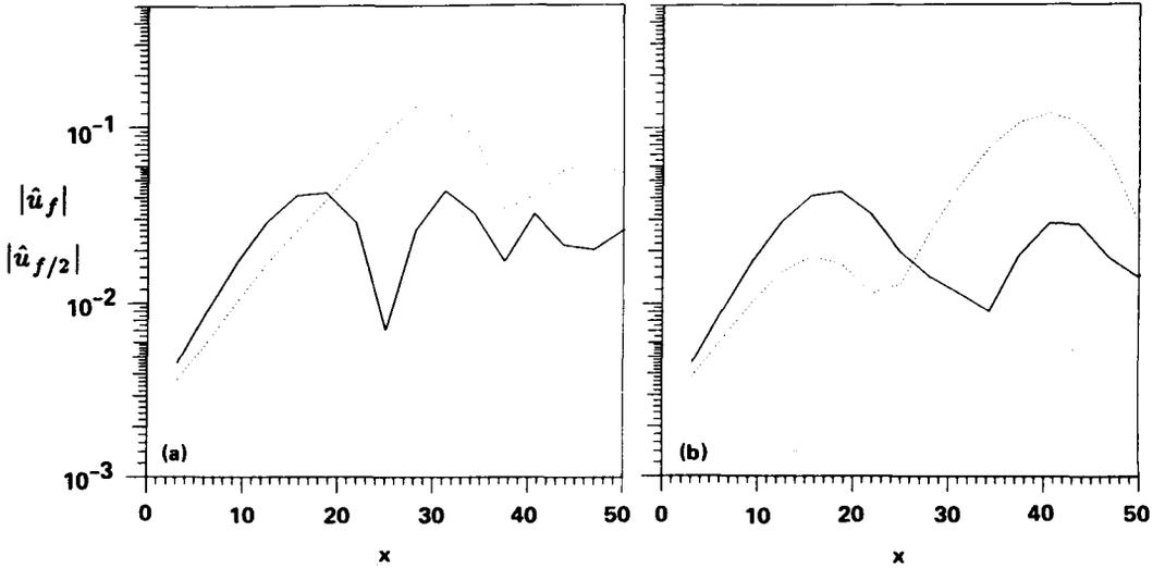
FIGURE 8. Development of  $|\hat{u}_f|$  and  $|\hat{u}_{f/2}|$  in the downstream direction at  $y = 0$ . a) Case 3, forcing the fundamental and its subharmonic with  $\phi = 0^\circ$ . b) Case 4, forcing the fundamental and its subharmonic with  $\phi = 90^\circ$ . —  $|\hat{u}_f|$ . .....  $|\hat{u}_{f/2}|$ .
