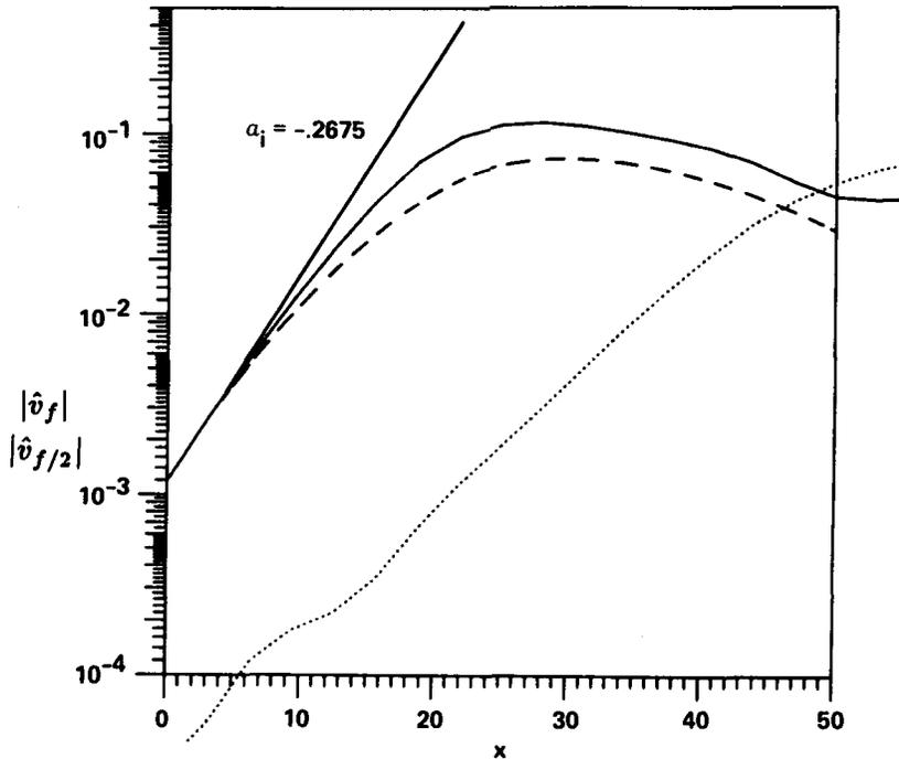
FIGURE 5. Effect of the Reynolds number on the development of the fundamental. —  $|\hat{v}_f|$  with  $Re = 600$ . ----  $|\hat{v}_f|$  with  $Re = 300$ . .....  $|\hat{v}_{f/2}|$  with  $Re = 600$ .
