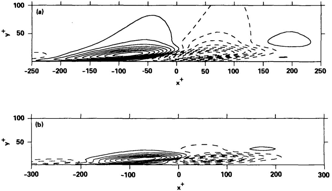
FIGURE 2. Contours of streamwise perturbation velocities in the plane  $z = 0$  for model VITA-educed coherent structure at  $\tau = 0$  ( $t^+ = 24$ ) for a variance integration time of  $T^+ = 20$ , with  $l_1 = 95$ ,  $l_2 = 15$ ,  $l_3 = 35$ . a) Flat-eddy approximation. b) "Sausage" approximation.
