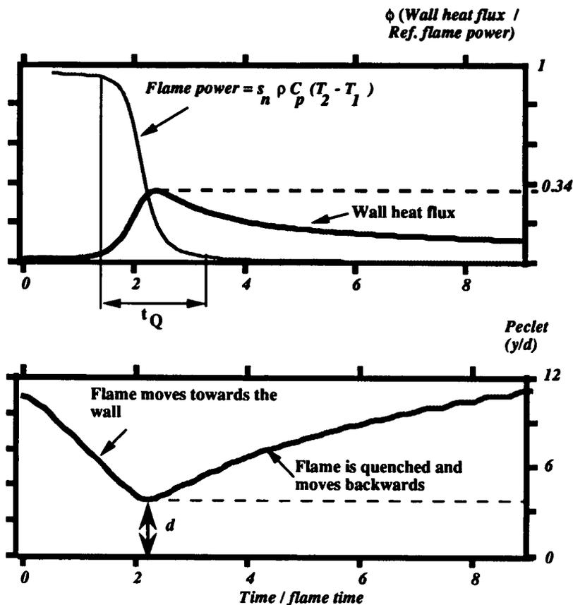
FIGURE 2. Numerical results for a laminar flame-wall interaction.
