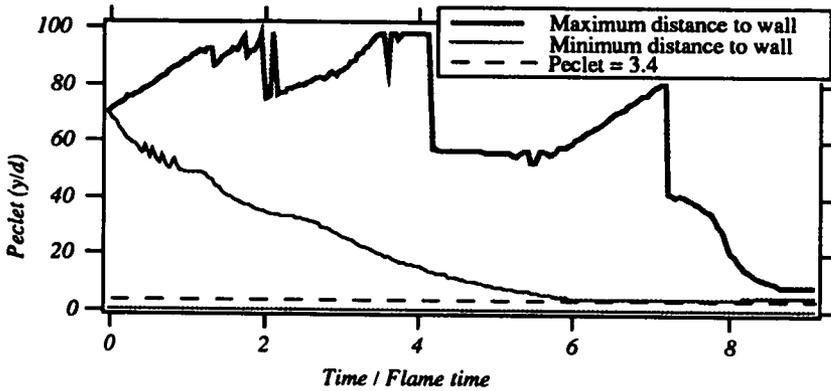
FIGURE 5. Maximum and minimum (over all computational cells adjacent to the wall) flame-wall distances for Case 2D4.
