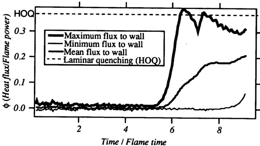
FIGURE 6. Minimum, maximum, and mean (over all computational cells adjacent to the wall) wall heat fluxes for Case 2D4.
