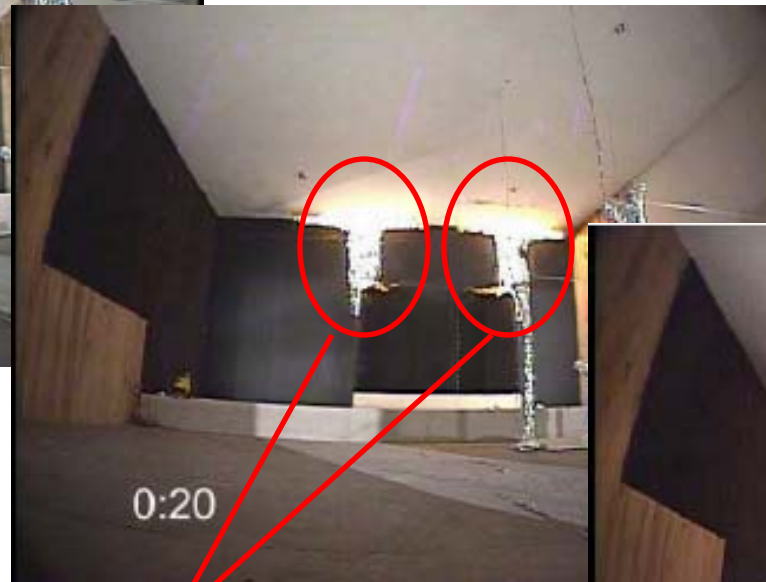
Vertical wall flames impinging on ceiling
