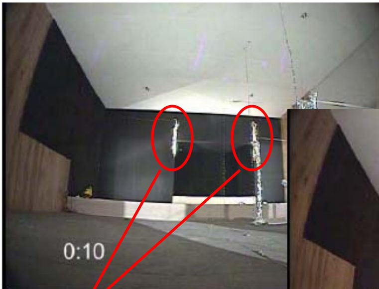
Ignition and early vertical spread of wall flames
