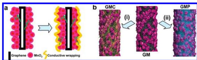
**Figure 1.** (a) Schematic illustration showing conductive wrapping of graphene/MnO<sub>2</sub> (GM) to introduce an additional electron transport path (in a discharge cycle). (b) Schematic of graphene/MnO<sub>2</sub>/CNT (GMC) and graphene/MnO<sub>2</sub>/conducting polymer (GMP) systems formed by wrapping of GM nanostructures with CNTs or conducting polymers (black, graphene; rose, MnO<sub>2</sub>; yellow, CNTs; blue, conducting polymer).
