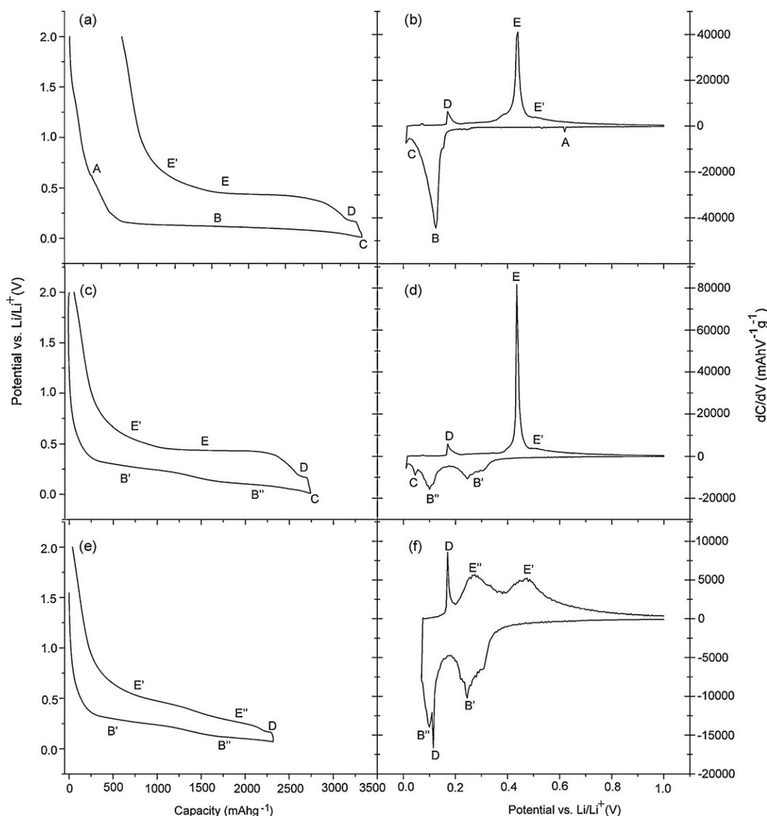
**Fig. 2.** Electrochemical potential spectroscopy data. Voltage profile (a) and differential capacity curve (b) of the first cycle, starting from crystalline SiNWs and charging to 10 mV. After the first cycle, the SiNWs turned amorphous, resulting in a different voltage profile (c) and differential capacity curve (d). Stopping the charge at 70 mV results in yet another different voltage profile (e) and differential capacity curve (f).
