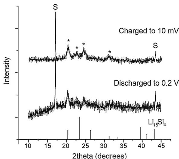
**Fig. 3.** X-ray diffraction data of SiNWs charged to 10 mV and discharged to 2.0 V. The peaks marked by S are from the stainless steel substrate. The peaks marked with \* are from the PEEK dome on the sample stage. The  $\text{Li}_{15}\text{Si}_4$  peaks, which are overlaid as a reference, do not appear in the scans.
