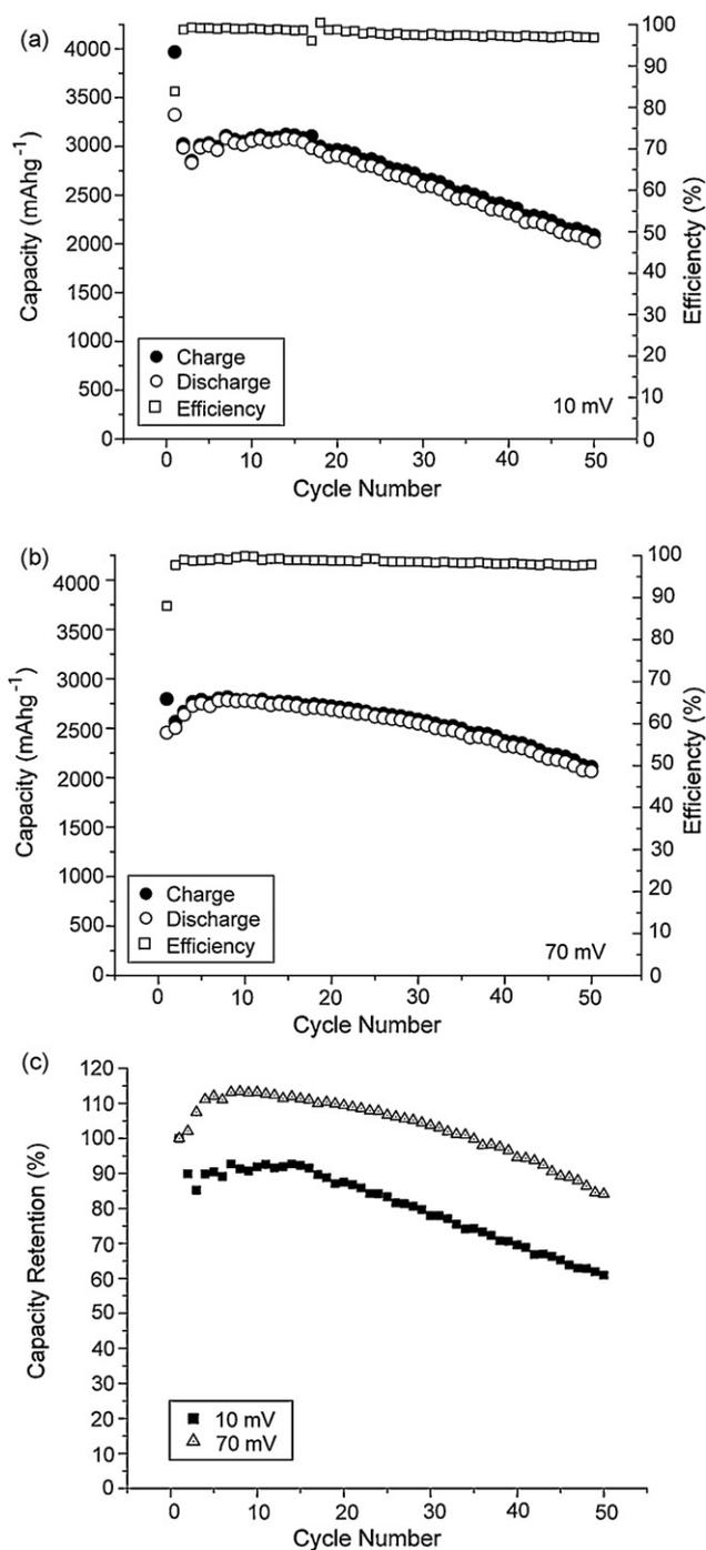
**Fig. 5.** Cycle life of SiNWs cycled at (a) C/5 rate with charge to 10 mV, (b) C/5 rate with charge to 70 mV and (c) the discharge capacity retention for the samples charged to 10 mV compared to 70 mV.
