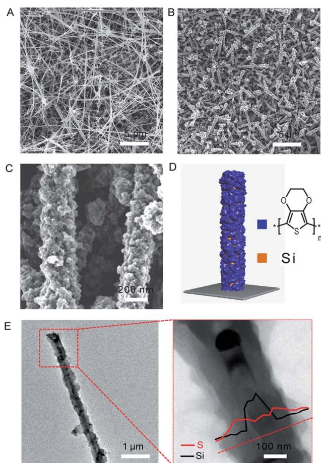
**Fig. 1** (A and B) Top view SEM images of pristine Si NWs and PEDOT-coated Si NWs. Scale bar:  $5 \mu\text{m}$ . (C) Magnified SEM image of PEDOT-coated Si NWs. (D) Schematic of a PEDOT (blue)-coated Si NW (brown) with the molecular structure of PEDOT shown. (E) TEM images of an individual PEDOT-coated Si NW. The EDX line scan profile shows the sulfur signal from PEDOT (red) and the Si signal from the core (black).
