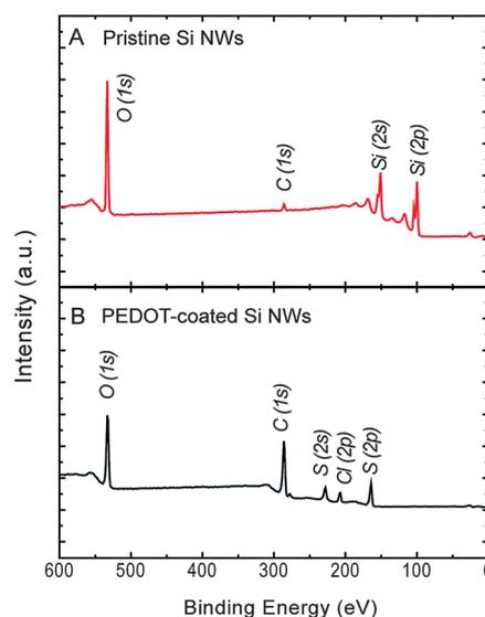
**Fig. 2** XPS characterization of PEDOT-coated Si NWs. (A) Pristine Si NW sample, (B) PEDOT-coated Si NW sample. The S signal is from PEDOT. No Si peaks were observed, which indicates the uniform and complete coverage of PEDOT on the Si NWs.
