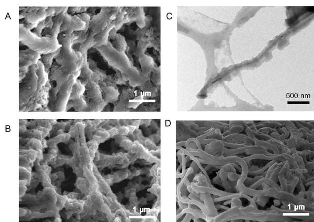
**Fig. 4** Characterization of Si NW anodes after 40 charge–discharge cycles. (A) SEM image of PEDOT-coated Si NW anode with SEI. (B) SEM and (C) TEM image of PEDOT-coated Si NW anode with SEI removed by dipping in 0.5 M HCl, showing that the PEDOT coating remains on the surface of the Si NWs. (D) SEM image of non-coated Si NW anode with SEI removed.
