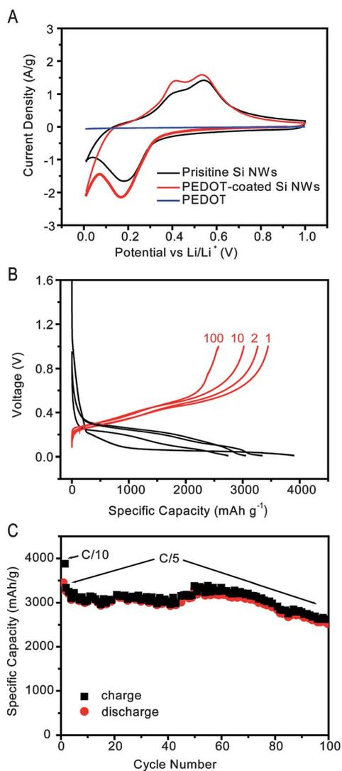
**Fig. 3** Electrochemical characterization of PEDOT-coated Si NW anodes. (A) Cyclic voltammetry (2<sup>nd</sup> cycle) of pristine Si NWs, PEDOT-coated Si NWs and a pure PEDOT electrode. (B) Galvanostatic charge–discharge voltage profile of PEDOT-coated Si NWs for the 1<sup>st</sup>, 2<sup>nd</sup>, 10<sup>th</sup> and 100<sup>th</sup> cycle. (C) Specific capacity with cycling of PEDOT-coated Si NWs. The first cycle is at C/10 and the remaining cycles are at C/5 (1C = 4200 mA g<sup>-1</sup>).
