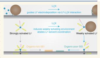
environment by decreasing Li<sup>+</sup>-solvent coordination, induces organic-poor SEI on the Li metal anode, and facilitates Li<sup>+</sup> transport in the electrolyte. Importantly, recognizing specific roles of SEI inorganics for Li metal anodes can serve as one of the rational guidelines to design and optimize SEIs through electrolyte engineering for LMBs.
