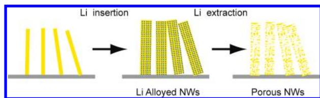
**FIGURE 1.** Schematic illustration of pore generation by the alloying/dealloying process. As-grown single-crystalline zinc oxide nanorods or silicon nanowires expand upon electrochemical Li ion insertion. As Li ions are extracted from these 1D nanomaterials, the nanostructures shrink but to volumes larger than the original. The increased volumes suggest pore formation inside the nanostructures.
