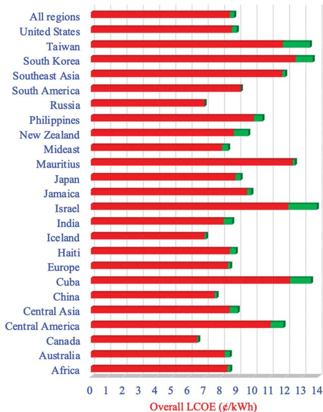
Fig. 4 Sensitivity of the overall 2050 levelized cost of energy (LCOE) with WWS, in 2020 USD, to a 50% higher battery cost (\$90 instead of \$60  $\text{kW}^{-1} \text{h}^{-1}$ -electricity storage). Red is the baseline cost (Table 4). Green is the incremental cost due to higher-cost batteries.
