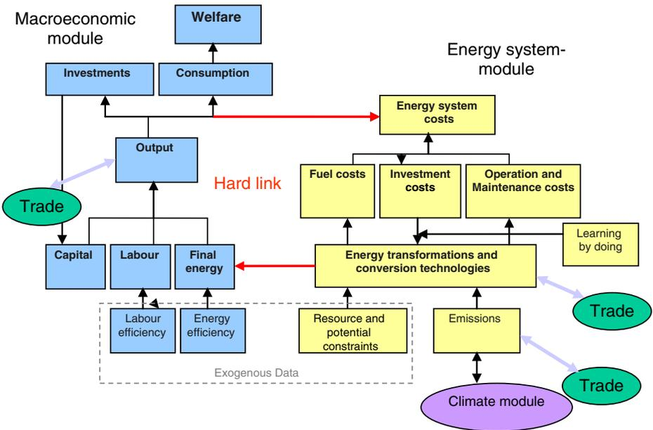
**Fig. 2** Overview of the REMIND-R model framework. Blue boxes on the left are related to the macroeconomic growth model, yellow boxes on the right denote elements of the energy system model. The red arrows highlight the hard-links between models. The light-colored arrows indicate trade relationships
