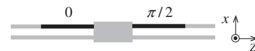
FIG. 4. The structure for experimental realization of the photonic Aharonov-Bohm effect. The gray regions are dielectric waveguides. The two black regions are modulated, with modulation phases of 0 and \pi/2 , respectively.
