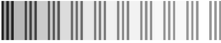
FIG. 1. View of the structure considered in this paper. Wide cavities of equal thicknesses d_{cav}=541 nm are separated by distributed Bragg mirrors which assemble five layers of thicknesses d_a=135 nm (clear) and d_b=100 nm (dark). The whole structure contains n wide cavities (our calculations use n=20 ), and n+1 mirrors. The refractive index (increasing with darker gray shades) of these layers is not periodic, but gradually modified along the depth of the structure.
