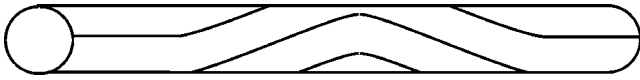
Fig. 1. Configuration of a single full twist applied to a length of fiber to alter the polarization of the signal at the fiber output end.
