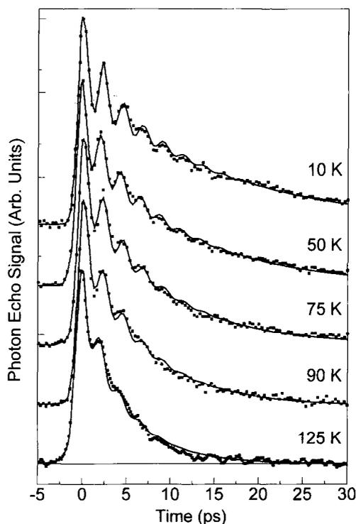
Fig. 1. Photon echo decays and fits for the asymmetric CO stretching mode of  $\text{W}(\text{CO})_6$  in di-butylphthalate at several temperatures in the glass. Fits are to Eq. (2) and represent the homogeneous dephasing of the three level coherence with beating at the anharmonic vibrational frequency splitting.
