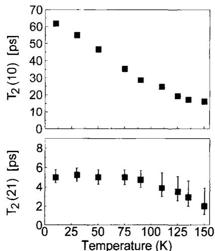
Fig. 2. Decay times  $T_2(10) = 1/\gamma_{10}$  and  $T_2(21) = 1/\gamma_{21}$  for temperatures between 10 K and 150 K obtained from fits to Eq. (2). Error bars for  $T_2(10)$  are on the order of the size of the squares. Error bars for  $T_2(21)$  show the influence of the small uncertainties in both  $T_2(10)$  and  $\Delta$  on the accuracy of the determination.
