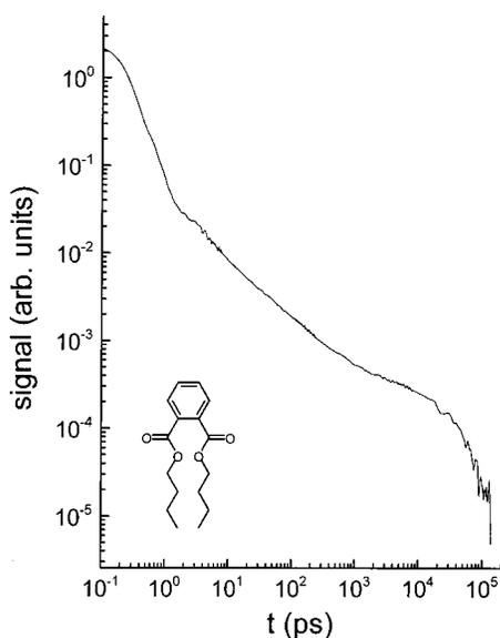
FIG. 1. Optical heterodyne detected optical Kerr effect data taken on supercooled dibutylphthalate at 234.0 K. The data are displayed on a log plot. The data span  $\sim 5$  decades in amplitude and 6 decades in time from 100 fs to 100 ns. The data decay approximately as an exponential at long time. At shorter times, two regions that decay as power laws can be identified. The inset shows a molecular diagram of dibutylphthalate.
