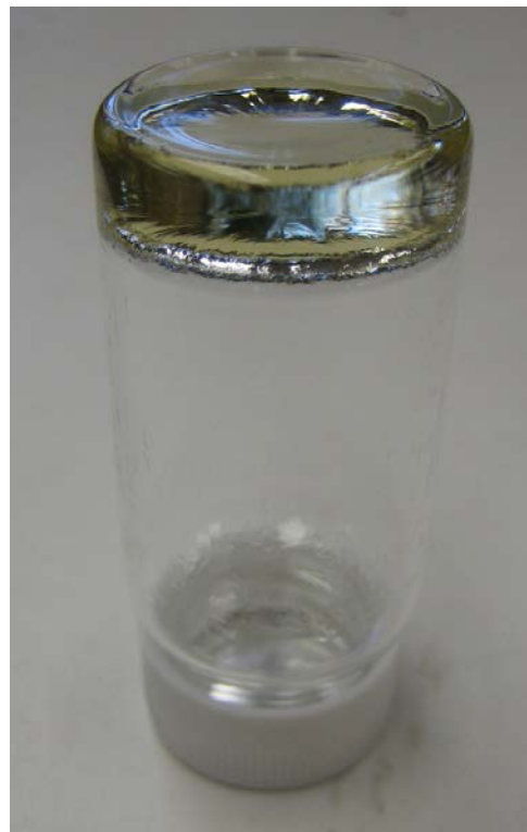
Figure 2. The figure shows a photograph of a sample vial with the OmimCl/water gel in which the vial has been inverted. The silver color is the reflection of light from the gel. The gel is stable for weeks and resists flow even when the sample vial is upside down as in the photograph.
