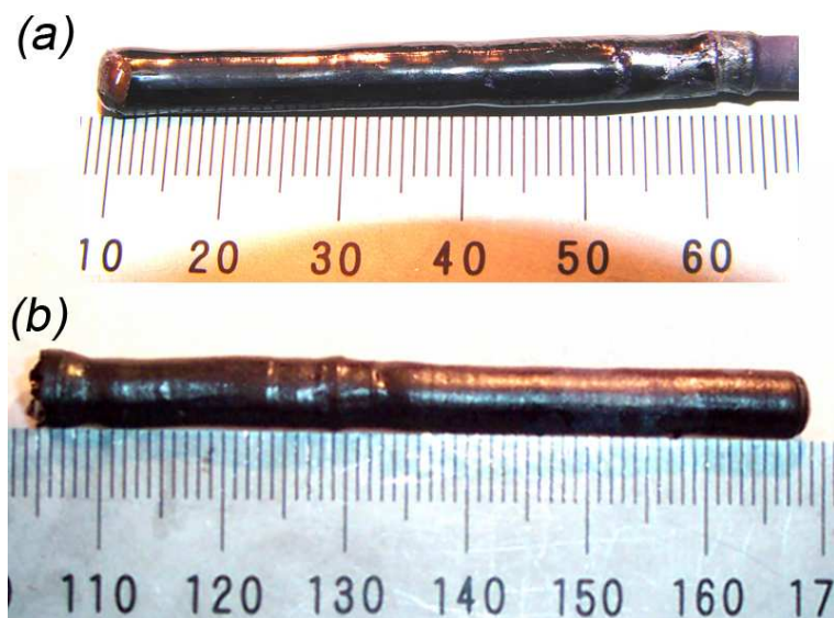
Figure 3.8. Typical single crystal grown using the travelling-solvent floating-zone technique in an image furnace (shown on a cm scale) (a) Sr_2Cu(BO_3)_2 (b) Ba_2Cu(BO_3)_2 .
