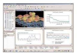
▲ C<sub>2</sub>H<sub>4</sub> absorption on Pt(111) surface. Electrostatic potential projected on the electronic density isosurface. Density of states, energy evolution, and energy convergence graphs.
