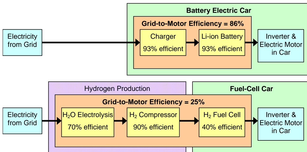
It is obvious that when we start with electricity (however it is produced), it is hard to beat the 86% efficiency of the currently available lithium-ion batteries and chargers. Even when we assume extremely high efficiencies for electrolysis, compression, and the fuel cell, the fuel-cell car requires more than three times as much electricity from the grid to drive the same distance.
