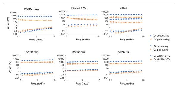
**Figure 3.** Rheological frequency sweep of storage (G') and loss (G'') moduli for various bio-inks. All bio-inks were tested at room temperature except for GelMA, which was measured at room temperature and 37 °C. PEGDA and GelMA bio-inks were cured by exposure to light ( $\lambda = 400-410\,$  nm) for 5 min RAPID inks were cured by exposure to a 10 mM calcium chloride solution for 10 min.
