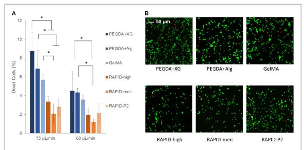
**Figure 5.** Cell print viability assay. (A) Quantification of LIVE/DEAD staining of 3T3 cells printed through a 32-gauge nozzle at average speeds of 75 and 60  $\mu$ l min<sup>-1</sup>. All bio-inks show less than 10% cell death during printing, while RAPID inks show less than 4% cell death. (B) Representative LIVE/DEAD confocal images of 3T3 cells printed at a flow rate of 75  $\mu$ l min<sup>-1</sup> immediately after print extrusion and before any curing steps.
