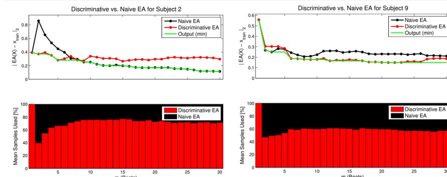
**Figures 5 and 6.** Discriminative EA increases the convergence rate compared to naive EA for typical Subject 2 (top, left) and 3 (top, right). Mean percentage of data used at each point in the corresponding discriminative EA (Bottom).
