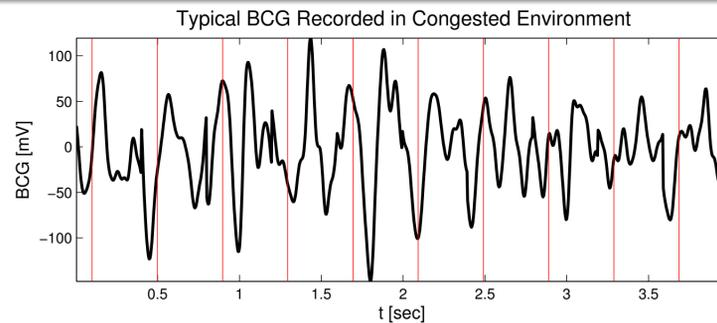
**Figure 2.** In a congested environment, BCG is difficult to distinguish because of the in-band noise that is much larger than the BCG component. The vertical red bars indicate ECG R peaks used to synchronize the ensemble.
