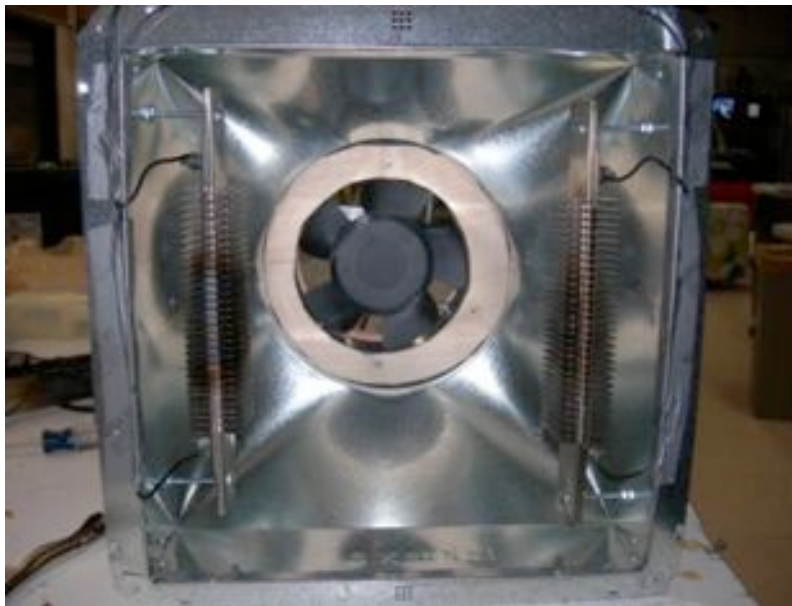
Figure 172: The electric heaters connected inside the air chamber of sub prototype 1
