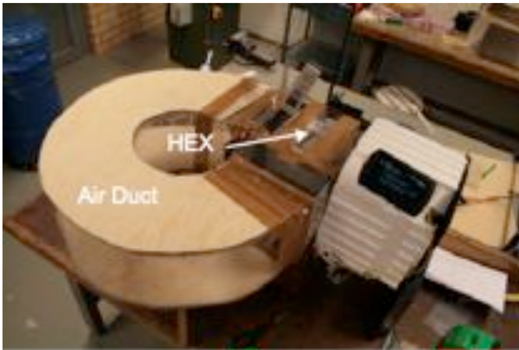
Figure 38: The final Pre-cooled VCC prototype. The ducts were added to divert the airflow through the Heat exchanger (HEX)
