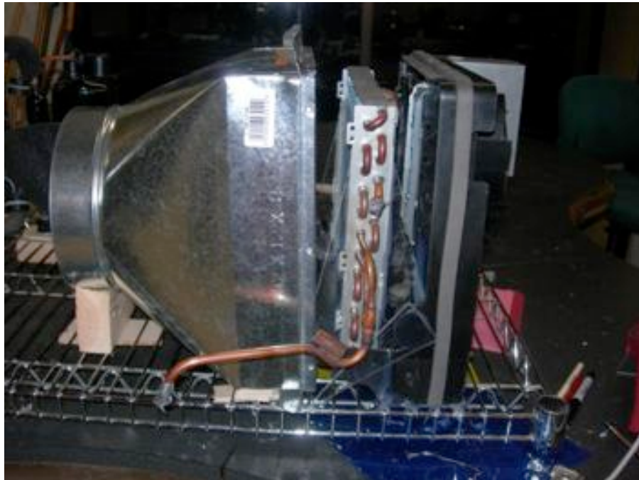
Figure 179: Close up of the evaporator and blower at the other end
