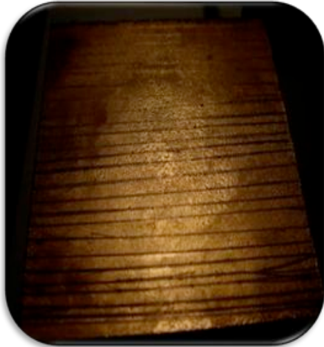
Figure 149: Experiment 5, moisture on scratched Copper shee
