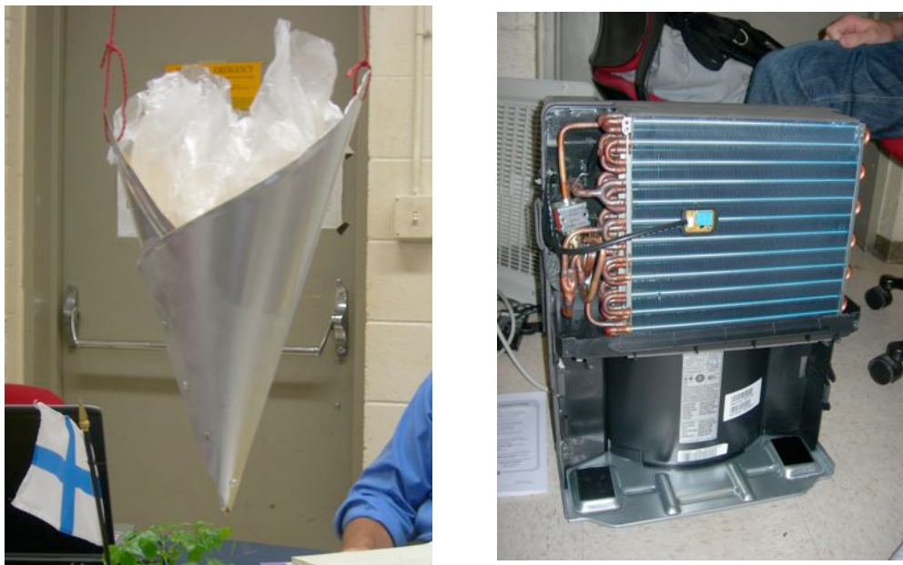
Figure 17: Condensing experiment and disassembly of Kenmore dehumidifier
