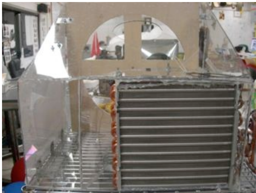
Figure 178: Condenser attached to the prototype - with the regenerative chamber and the wheel frame at the back
