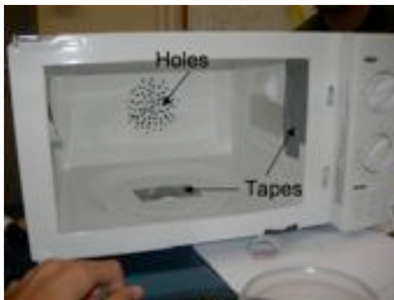
Figure 35: Holes drilled to the back wall for air flow and duct tapes used to close other holes inside the microwave
