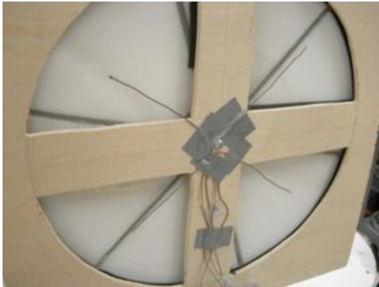
Figure 173: The thermocouple probes used to measure air temperature outside the desiccant wheel
