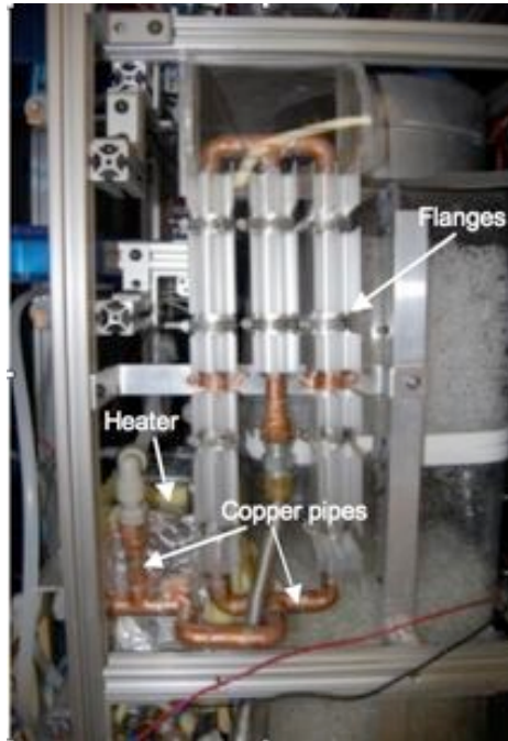
Figure 89: The Condenser system
