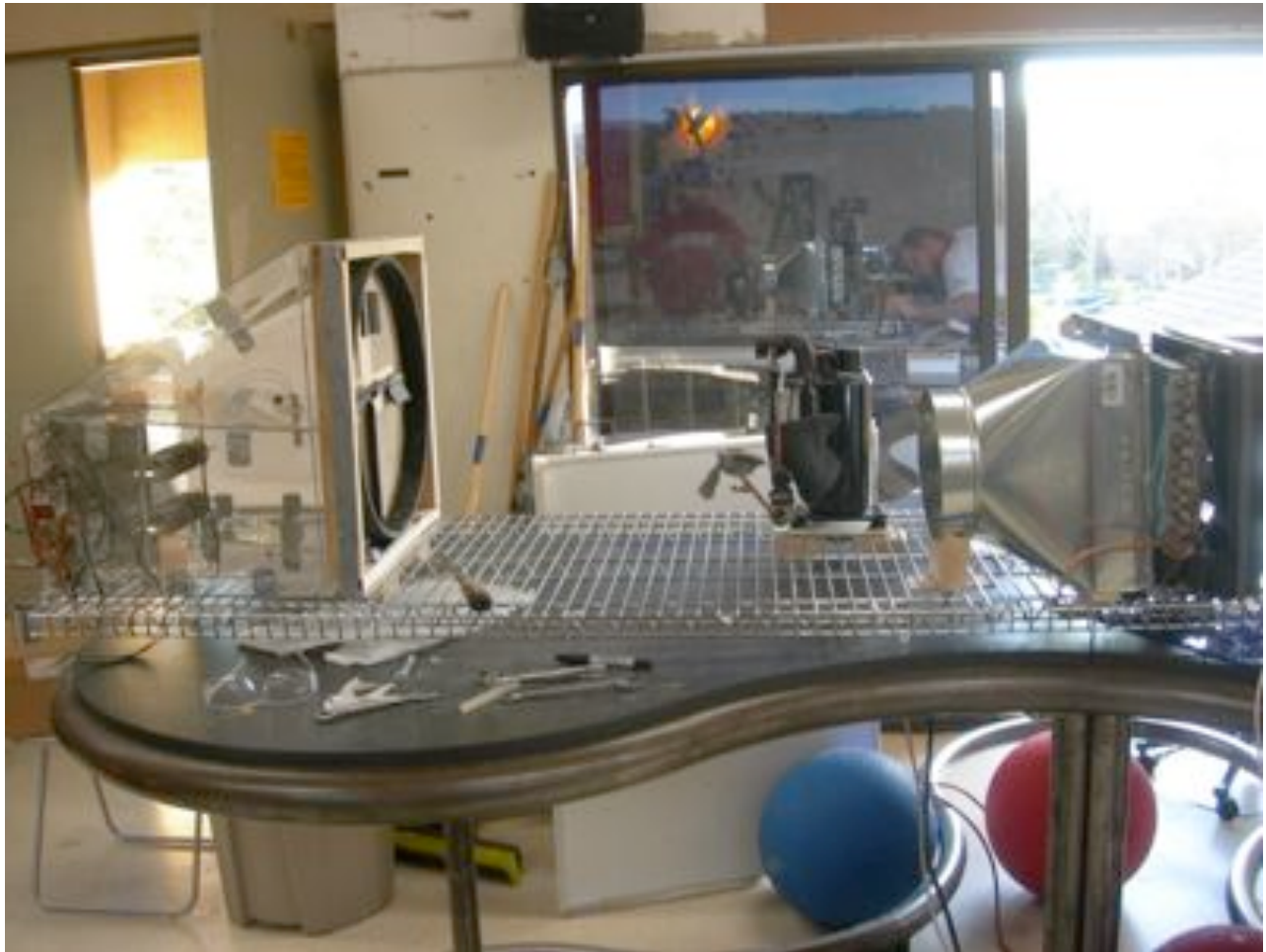
Figure 176: Desiccant Wheel-VCC Prototype as it stood before the reconnection of pipes - One can see the desiccant wheel frame on left with the required regenerative air ducts and heaters. The solo compressor stands in the middle. On the right is a part of the duct
