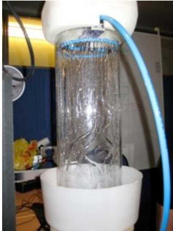
Figure 204: Plastic nozzle with holes
