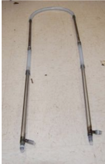
Figure 66: First prototype tube-in-tube heat exchanger. Inlet and outlet can be seen in the foreground.
