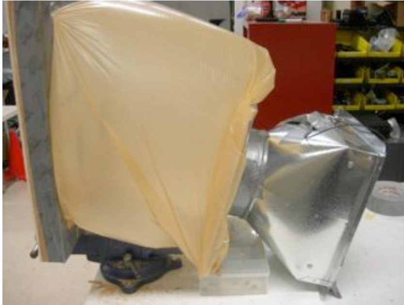
Figure 171: Prototype 1: The objective was to test the desiccant wheel efficiency
