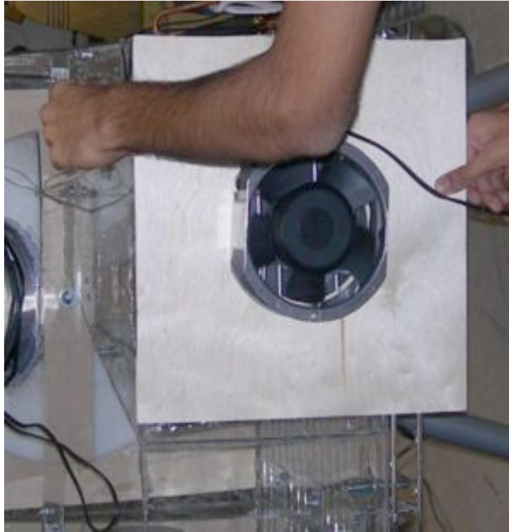
Figure 185: Extra fan added to cool the condenser
