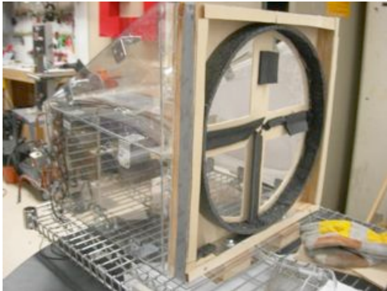
Figure 177: Close-up of the wheel frame with regenerative air chamber, heaters and condenser at the back
