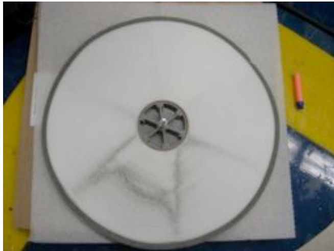
Figure 168: Desiccant Wheel used in the prototype
