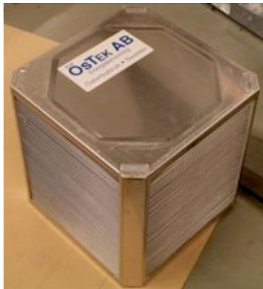
Figure 157: Cross flow heat exchanger used in the prototype
