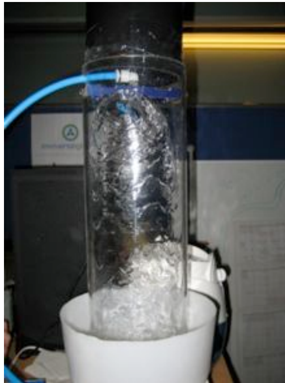
Figure 205: Rotating nozzle with openings on side
