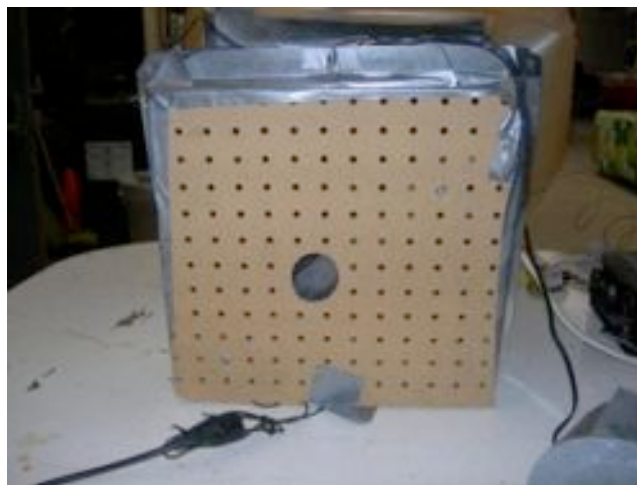
Figure 174: The contraption used to crudely control the air flow through the wheel
