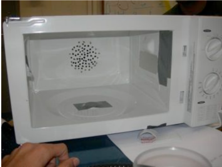
Figure 154: Holes drilled to the back wall for air flow. Duct tapes were used to close other holes inside the microwave (side walls and floor)
