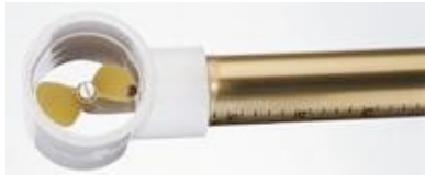
Figure 21. Air Velocity meter probe
