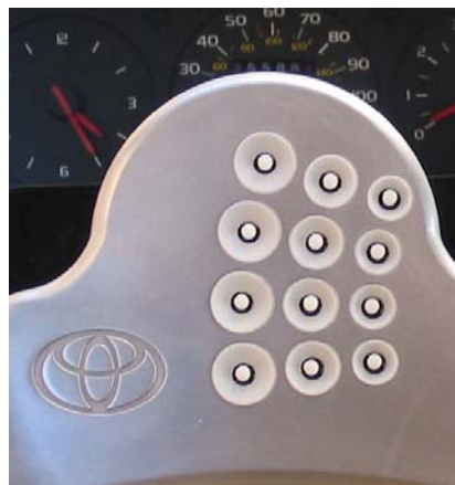
Fig. 20: Final button design with joysticks encompassed by inserts.
