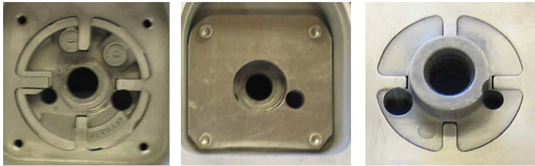
Fig. 25: Adaptor retained in steering wheel.
