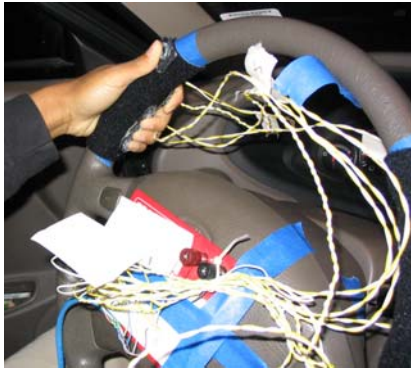
Steering wheel with buttons on front and back as used for CFP.
