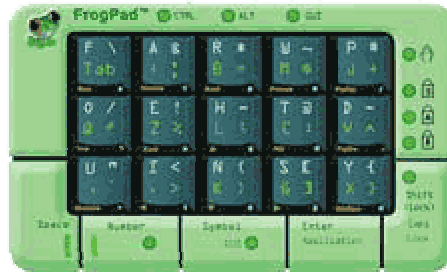
Fig. 64: Frogpad - a one handed input device
