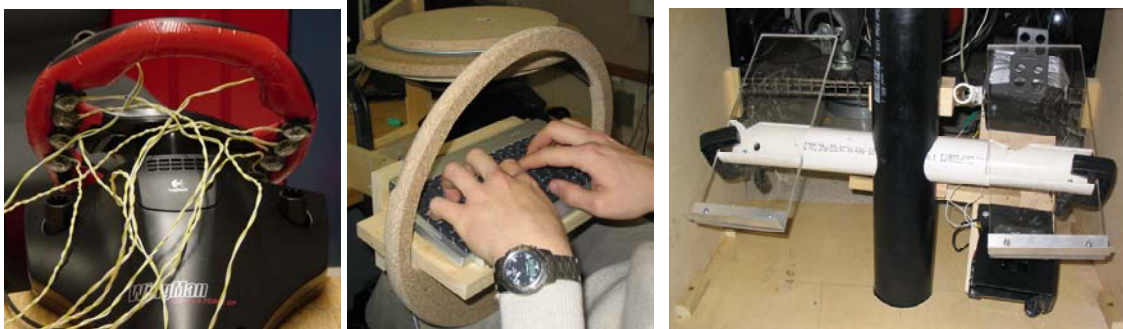
Critical (Buttons on Steering Wheel) and First Functional (QWERTY and Foot-Steering) Prototypes
