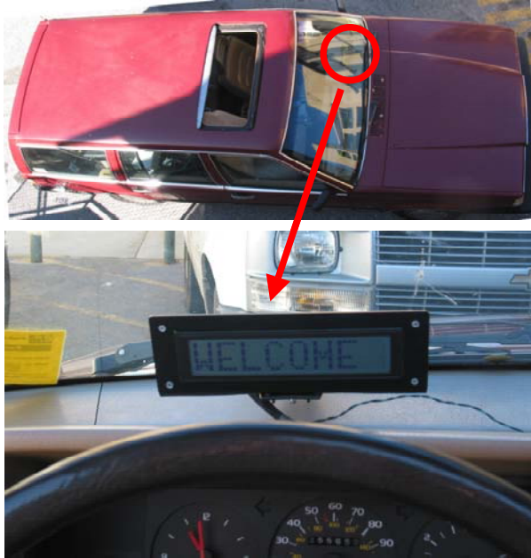
Fig. 85: LCD display below line of vision for limited character display
