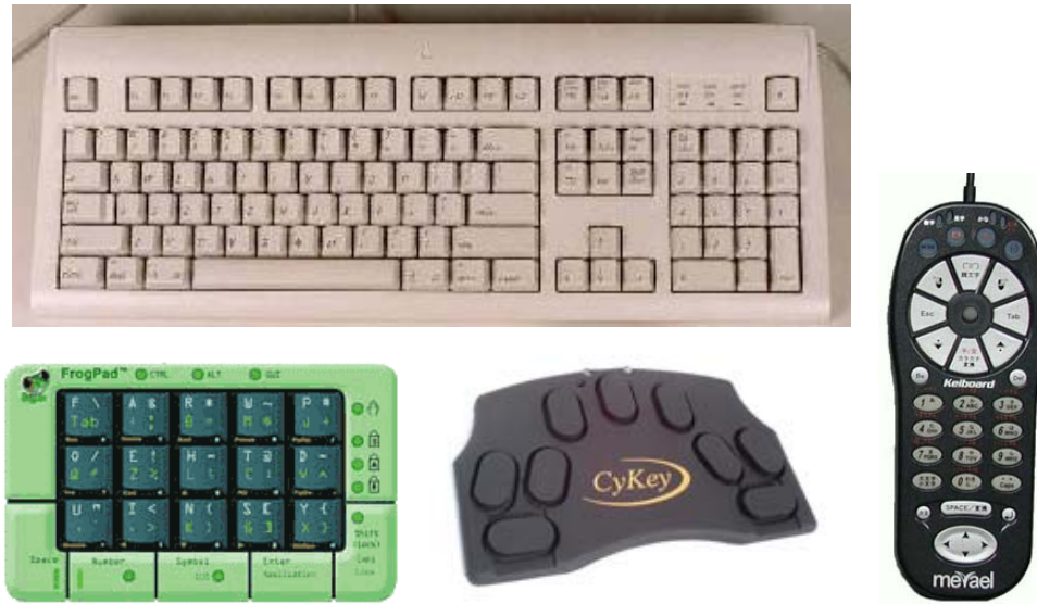
Fig. 5: Text input interfaces considered: QWERTY keyboard, Frogpad, CyKey and Keiboard.
