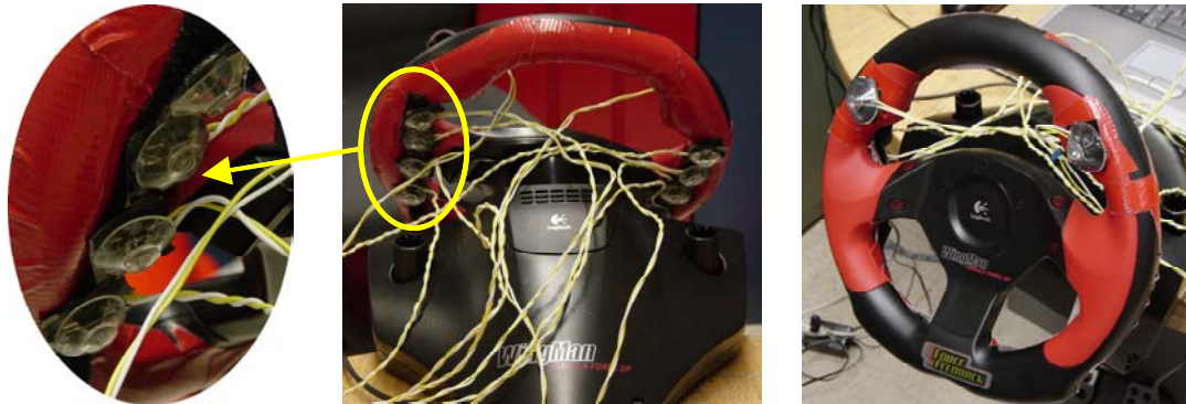
Fig. 77: Micro switches on front and back of simulator steering wheel
