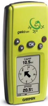
Fig. 37: GPS receiver used for speed measurement.
