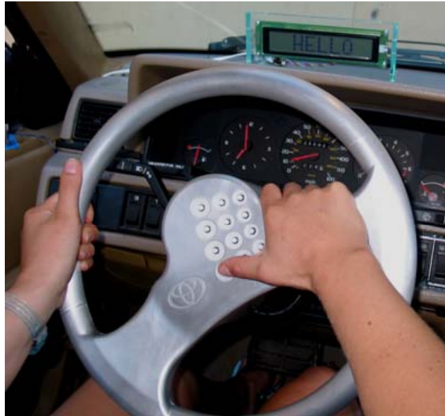
Fig. 21: Final design of optimum human-machine input interface steering wheel.
