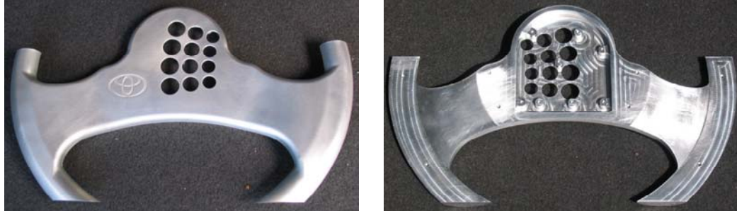
Fig. 27: Bezel part of final design.
