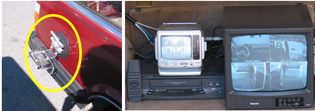
Fig. 38: Cameras on rear fenders and video recording system used to monitor lane departures.
