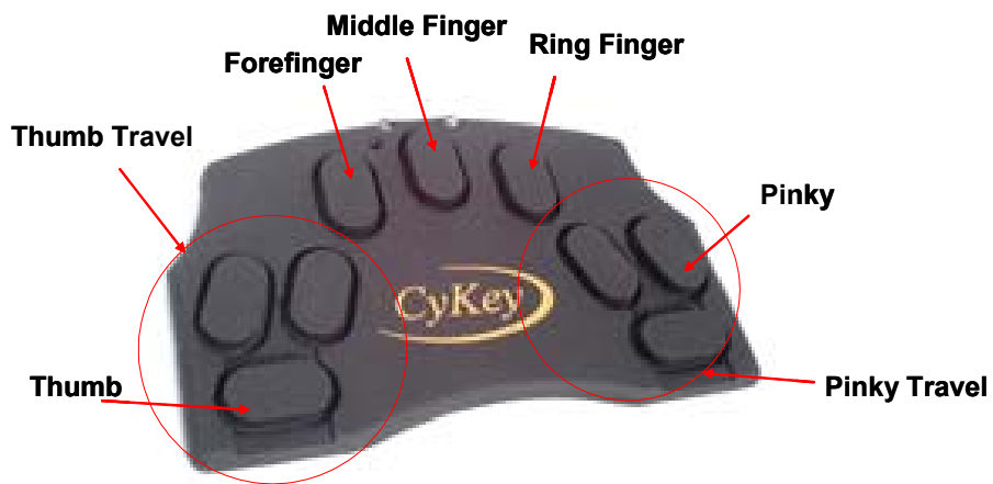
Fig. 66: The CyKey chorded-keyboard highlighted with the finger home positions and travel for right-handed use.
