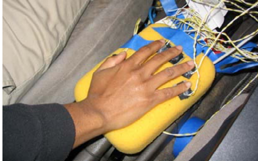
Fig. 79: Buttons on center console for one-handed input
