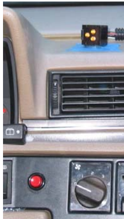
Fig. 35: LEDs and button used to measure reaction time.
