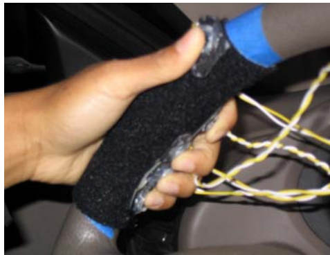
Steering wheel with buttons on front and back as used for CFP.
