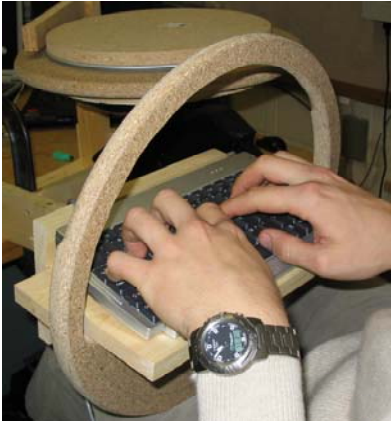
Prototype of steering wheel with integrated keyboard.
