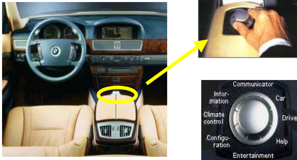
Fig. 58: BMW's I-Drive as used in the 7series 25
