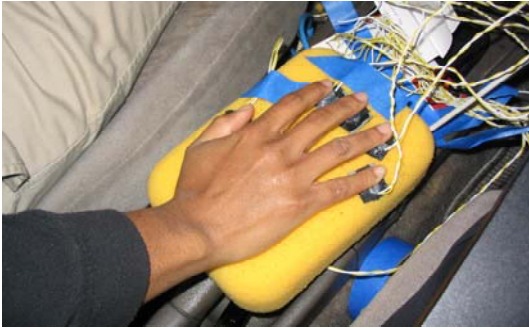
Buttons on center console for one-handed input.
