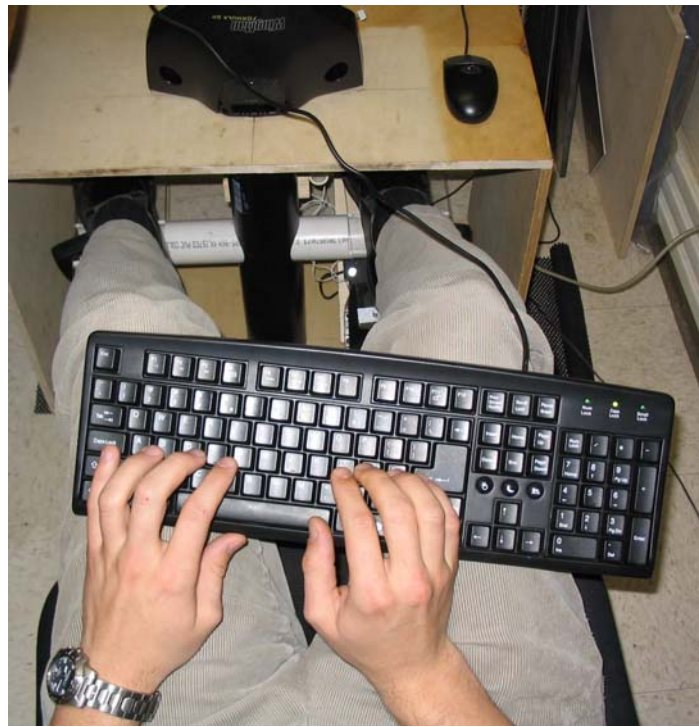
Picture of keyboard and foot steering system used in test.
