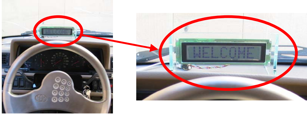
Fig. 31: LCD Display used for simulation of a heads-up-display.
