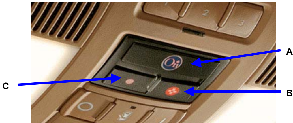
Fig. 62: OnStar interface in roof module of Audi A8 28
