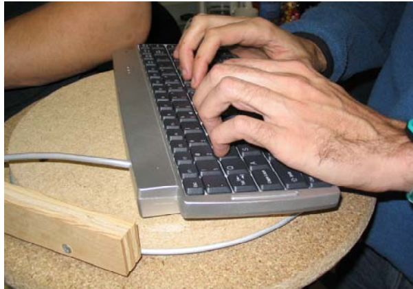
Prototype of steering wheel with integrated keyboard.
