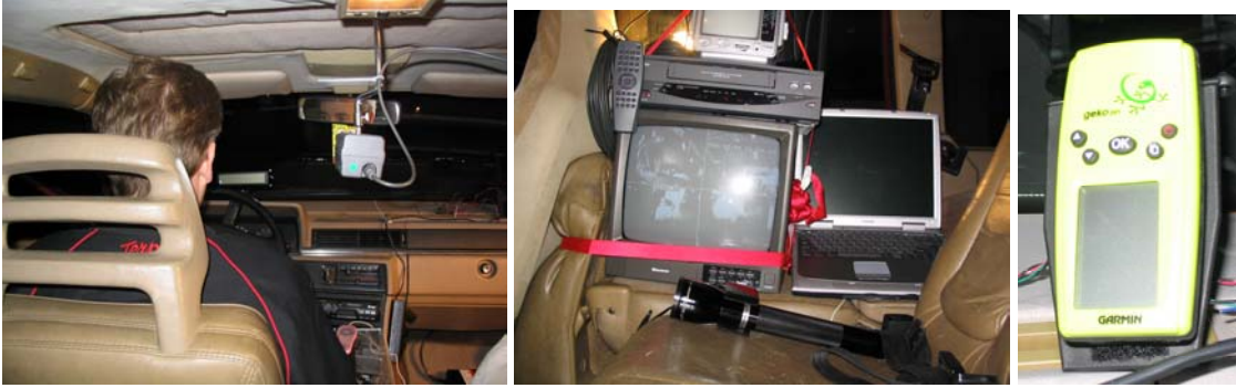
Camera to track driver, recording setup and GPS used to measure speed
