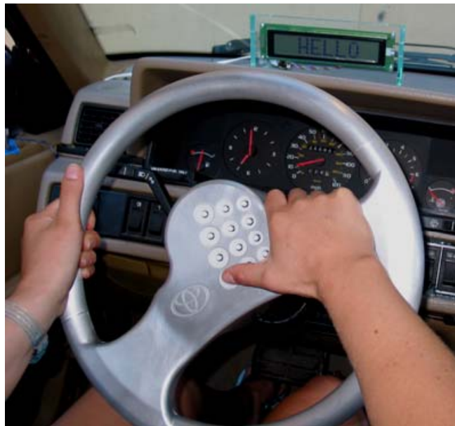
Fig. 1: The Optimum Human Machine Interface for text entry while driving.
