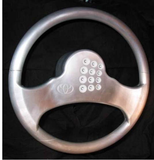
Fig. 4: Final design of a steering wheel with twelve buttons that can be activated in five directions to allow unique character mapping.
