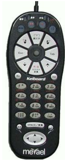
Fig. 67: Keiboard - One handed interface for use with the thumb
