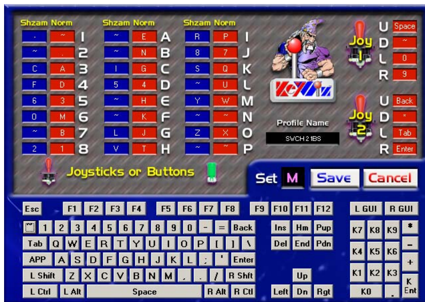
Fig. 49: Screenshot of KeyWiz software used to assign characters to 56 inputs of the KeyWiz Eco keyboard emulator.
