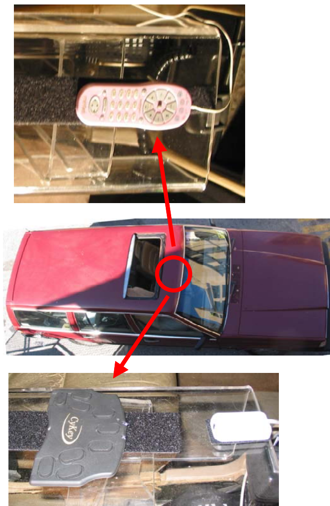
Fig. 84: Keyboard and CyKey mounted to center console
