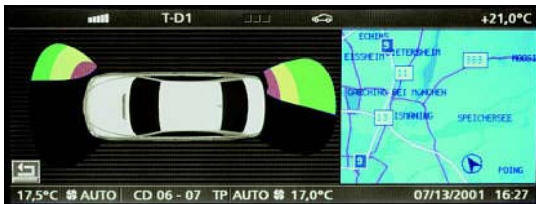
Fig. 59: BMW I-Drive split screen showing Park Distance Control and navigation map at the same time 26
