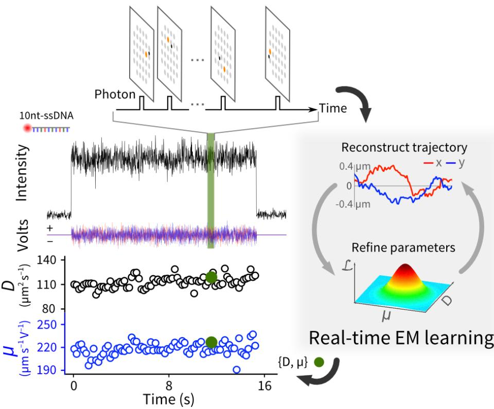
Statistical analysis of molecular motion in the ABEL trap yields estimates of single-molecule diffusion coefficient ( $D$ ) and electrokinetic mobility ( $\mu$ )
