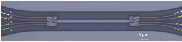
Fig. 1. Micrograph of four-channel back-to-back inverse-designed MDM multiplexer devices.
