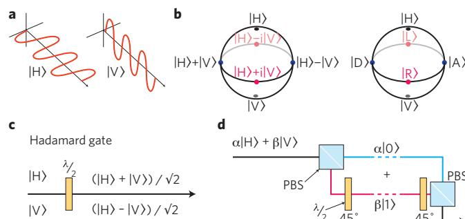
**Figure 1 | Encoding and manipulating a qubit in a single photon.**
