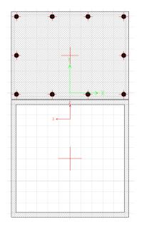
Inner ring beams  $\rightarrow$  HSS16x12x5/8  $\rightarrow$  12"x12" Concrete
