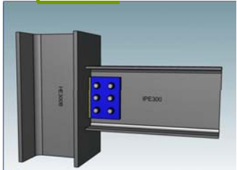
-Typical connection details
