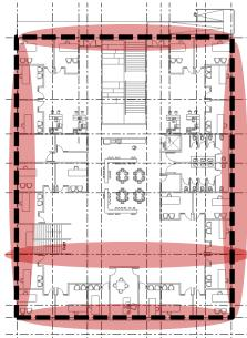
• Perimeter Trusses integrated into the façade
