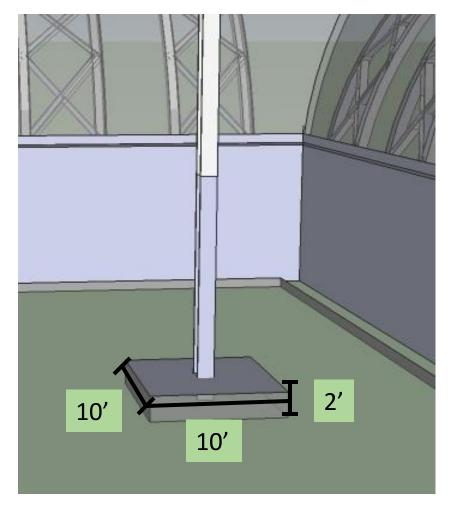
Spread Footing- Normal Weight Concrete 10 #9s in each direction (Mentor Reference: Greg Luth)
