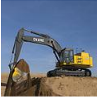
John Deere 330 LC 2.3 cu. Ft. Bucket 26.5' Max Dig Depth
