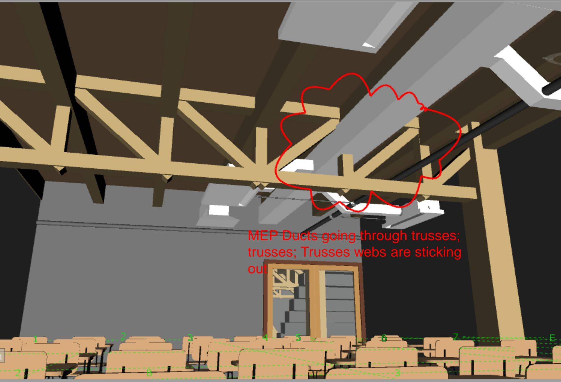
MEP Ducts going through trusses;
