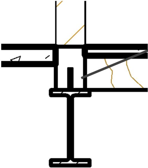
Pins on steel beams and core replacing columns
