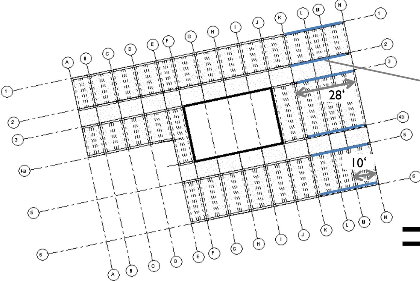
Steel beams holding up cantilever W 14x48
