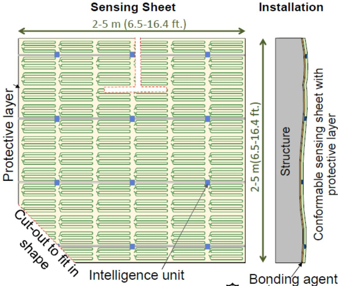
A nervous system for the building, with sensors detecting anomalous strains
