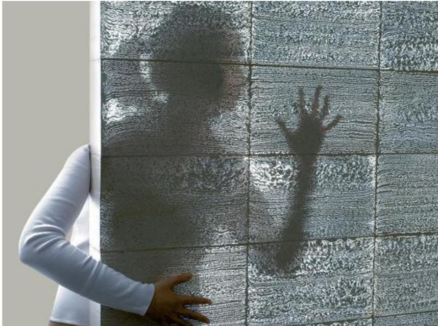
Use of translucent concrete to allow light in restrooms while maintaining structural integrity of shear walls (L-shape Concrete option)
