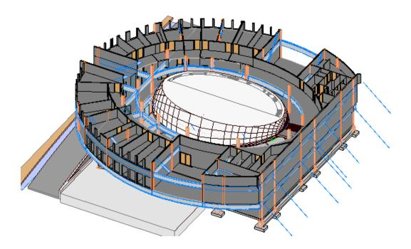
Column:W14X132 Girder: W24x94 @ Front Cantilever (Curved) Girder: W18x65 Other (Curved) Beam: W18x65 (Curved) Brace: W16x45 Composite Slab: 2" Deck + 4" Concrete Cover
