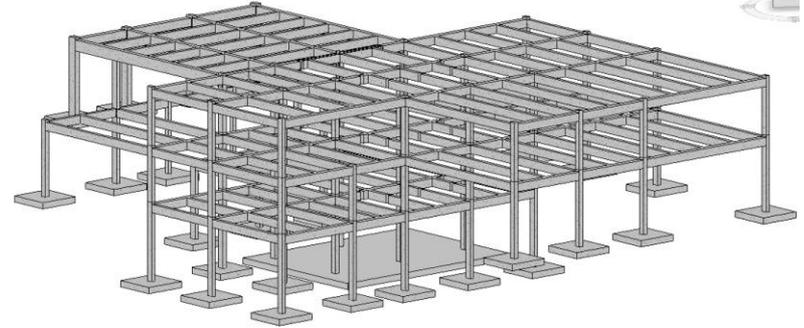
Glulam Beams and Concrete Columns
