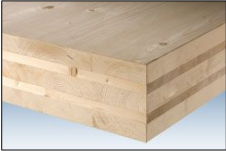
7 layer Top and bottom slab Depth = 6"
