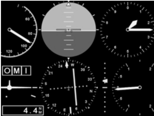
Figure 1. Conventional instrument suite used for control case
