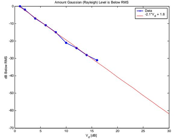
Fig. 8. Reduction of rms electric field value as a function of  $V_d$ .
