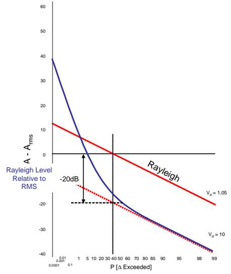
Fig. 7. Example of the rms reduction due to hole-punching for  $V_d = 10$ .
