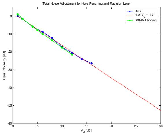
Fig. 9. Plot of total noise reduction as a function of  $V_d$  (blue). SSMA noise reduction due to clipping (green).
