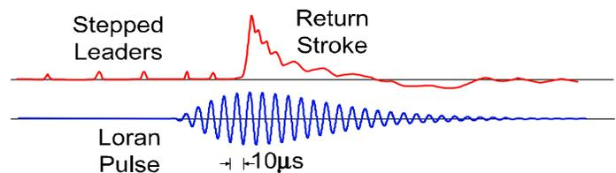
Fig. 1. Time history of a return stroke and a Loran pulse.
