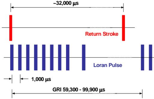
Fig. 2. Diagram of lightning and Loran pulse durations.
