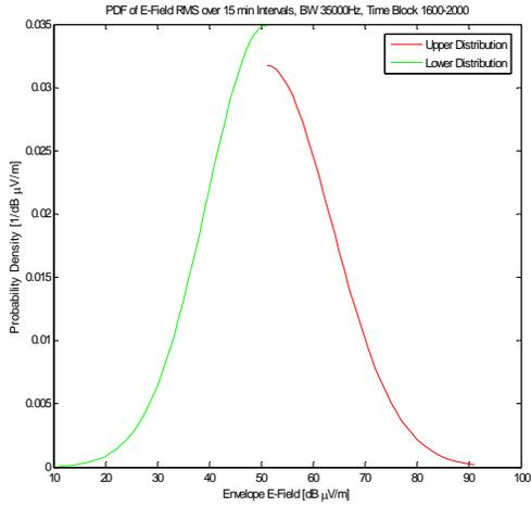
Figure 2: Probability Density Function for Summer 1600-2000h with 35kHz BW at 100kHz.
