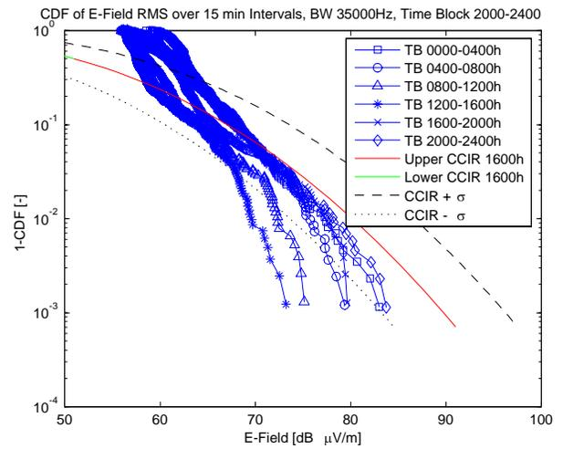
Figure 14: 1-CDF of the measured 35 kHz 15-minute averaged envelope rms values in all time blocks bounded by the CCIR estimation of the worst-case, 1600h time block, estimate.
