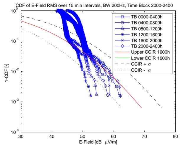
Figure 15: 1-CDF of the measured 200 kHz 15-minute averaged envelope rms values in all time blocks bounded by the CCIR estimation of the worst-case, 1600h time block, estimate.
