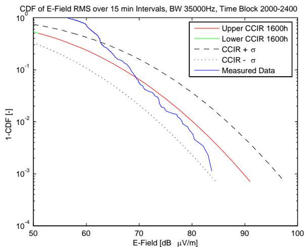
Figure 13: 1-CDF of the 35 kHz measured 15-minute averaged envelope rms values in the 2000h time block bounded by the CCIR estimation of the worst-case, 1600h time block estimate.
