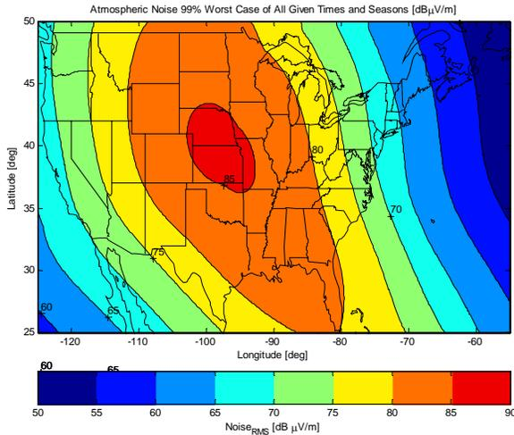
Figure 3: Median 99% noise level over all times and seasons for a 35kHz wide receiver centered at 100kHz.
