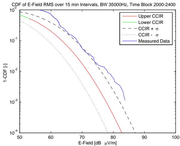
Figure 12: 1-CDF of the 35 kHz measured 15-minute averaged envelope rms values in the 2000h time block with the CCIR estimation of the same time block.
