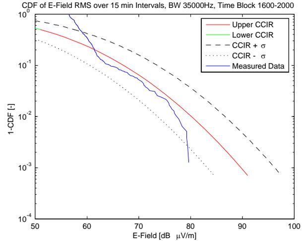
Figure 11: 1-CDF of the 35 kHz measured 15-minute averaged envelope rms values in the 1600h time block with the CCIR estimation of the same time block.
