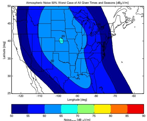
Figure 1: Median 50% noise level over all times and seasons for a 35kHz wide receiver centered at 100kHz.
