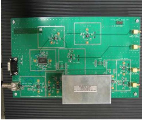
Figure 7: Atmospheric noise receiver for the Loran Band.
