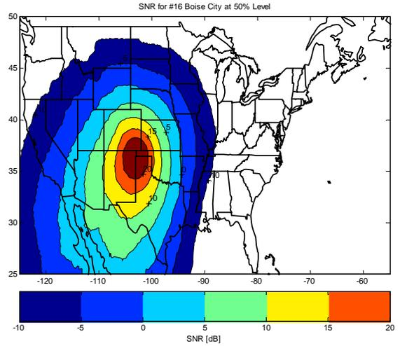
Figure 4: Boise City coverage given the median 50% noise level with a cut-off at SNR = -10dB.
