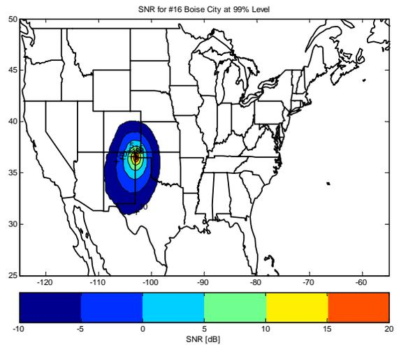
Figure 5: Boise City coverage given the median 99% noise level with a cut-off at SNR = -10dB.
