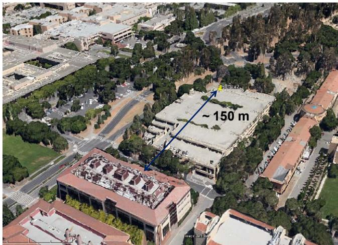
Figure 14. Potential Source of 1090 MHz Mode S Multipath (Site 2)
