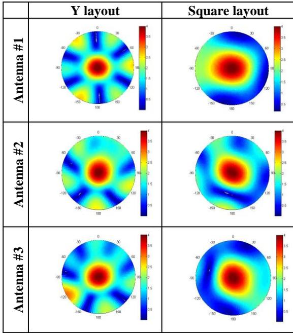
Figure 12. Patterns of three models of antenna and two layouts toward elevation 90 °
