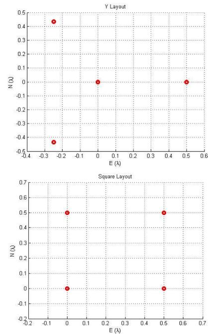
Figure 3. Physical layout of antenna array
