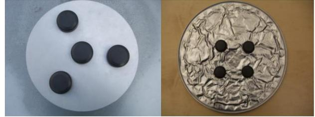
Figure 2. Photos of antenna array
