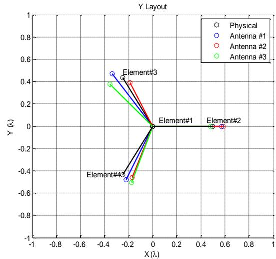
**Figure 10. Results of electrical layout using three models of antenna compared to physical layout for Y layout**
