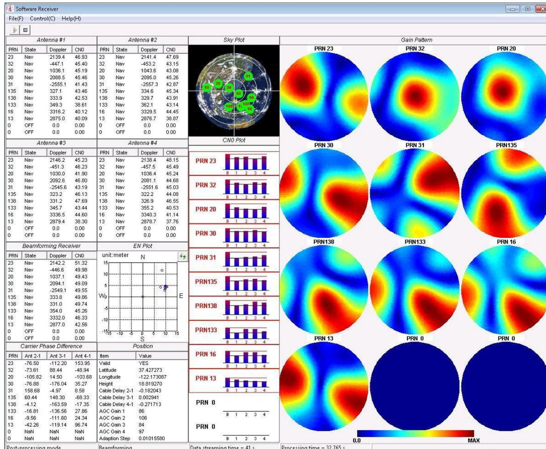
Figure 8. Screenshot of CRPA software receiver GUI
