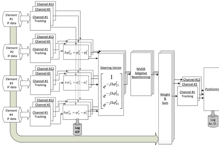
Figure 7. Block diagram of the software architecture
