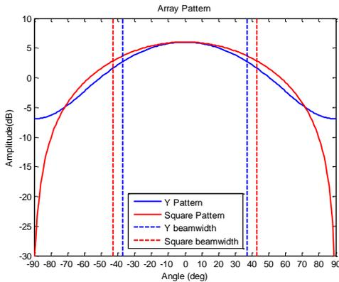
**Figure 4. Beamwidth of patterns of Y and square layouts (3 dB beamwidth shown)**
