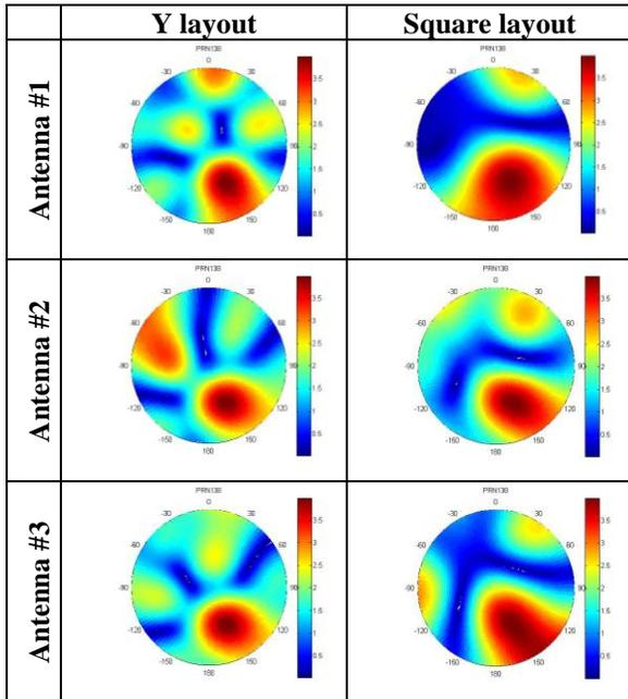
Figure 13. Patterns of three models of antenna and two layouts toward WAAS GEO PRN138
