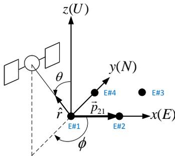
Figure 1. Antenna geometry and direction of satellite
