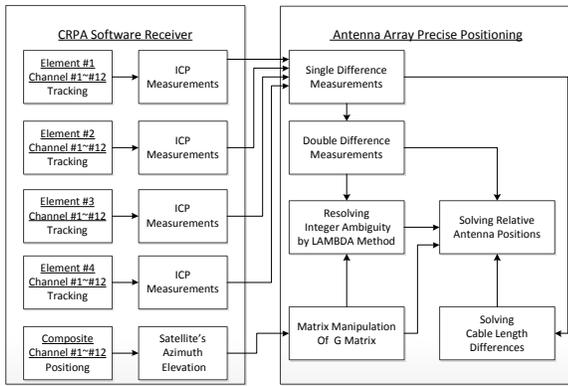
**Figure 9. Procedure of calculating antenna array electrical spacing**
