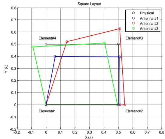
**Figure 11. Results of electrical layout using three models of antenna compared to physical layout for square layout**
