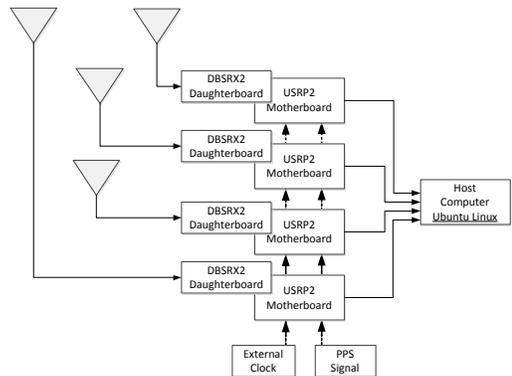
**Figure 5. Block diagram of the signal collection hardware**
