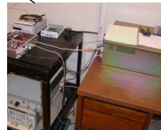
Data collection computer (2) ICS-650 cards sampling at 5-65 MHz and 12-bit A/D resolution
