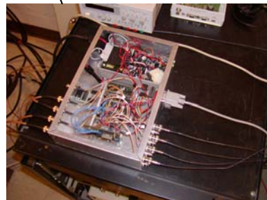
Analog front-end 4-channel GP2015 with 10 MHz common clock
